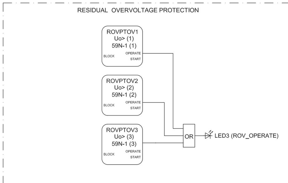
Figure 48: Residual overvoltage protection
