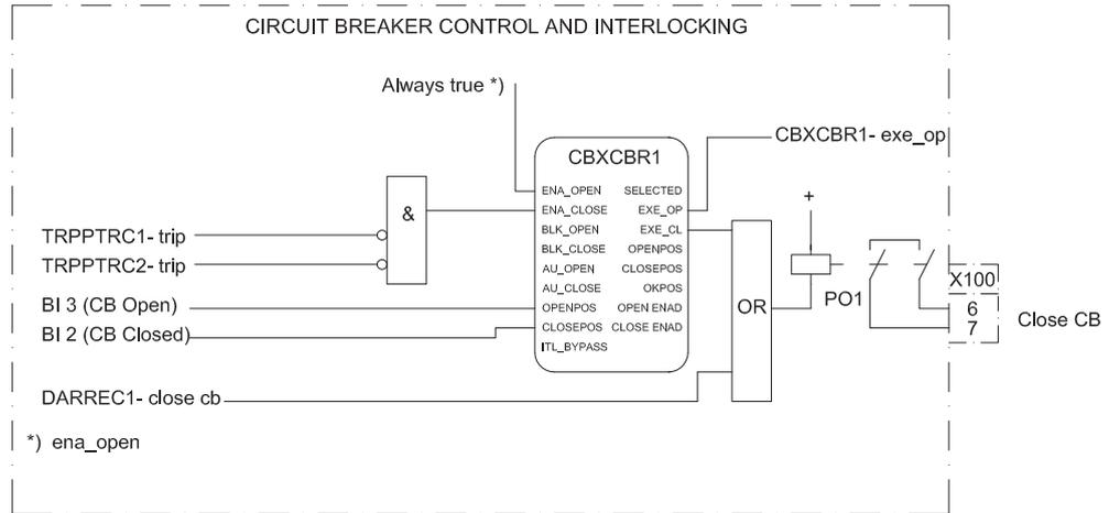
Figure 19: Circuit breaker control
