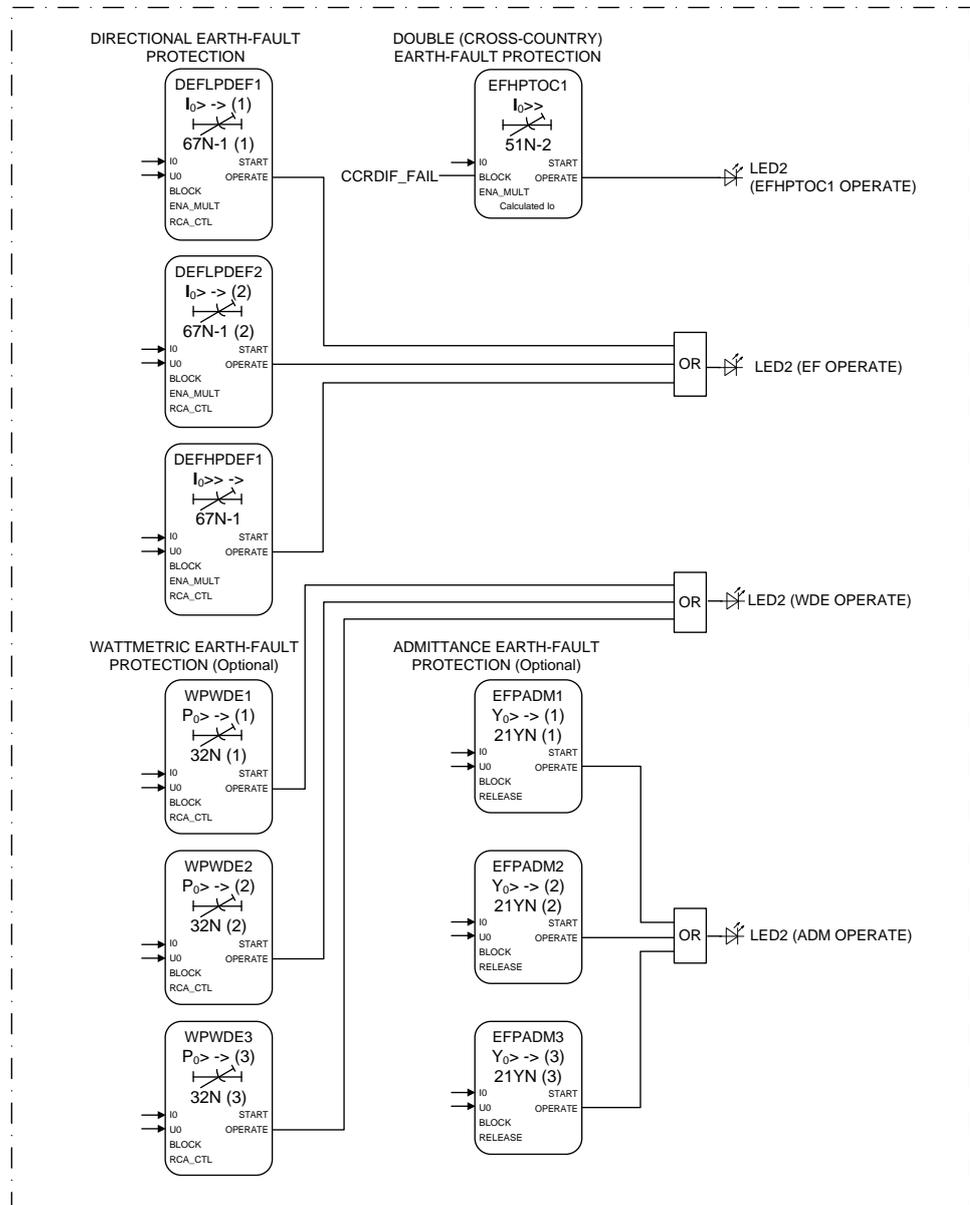
Figure 69: Directional earth-fault protection
