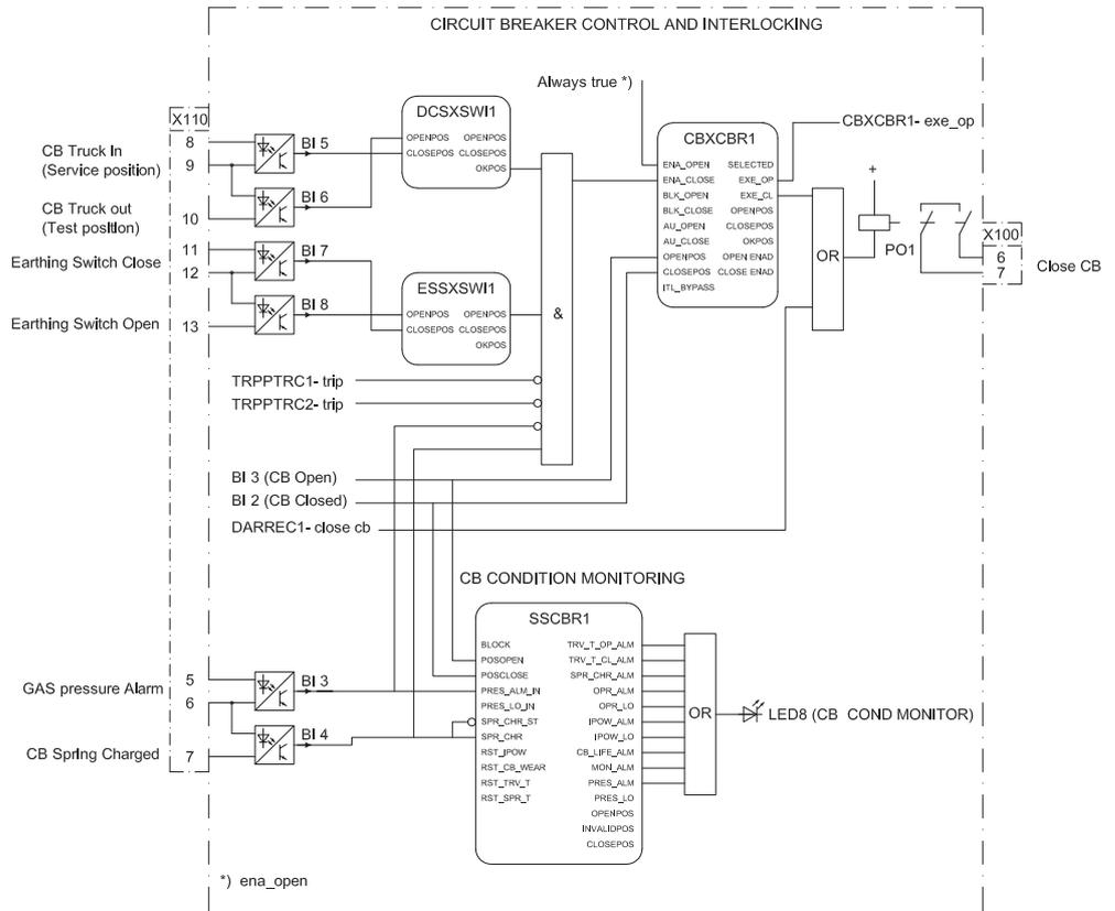
Figure 28: Circuit breaker control
