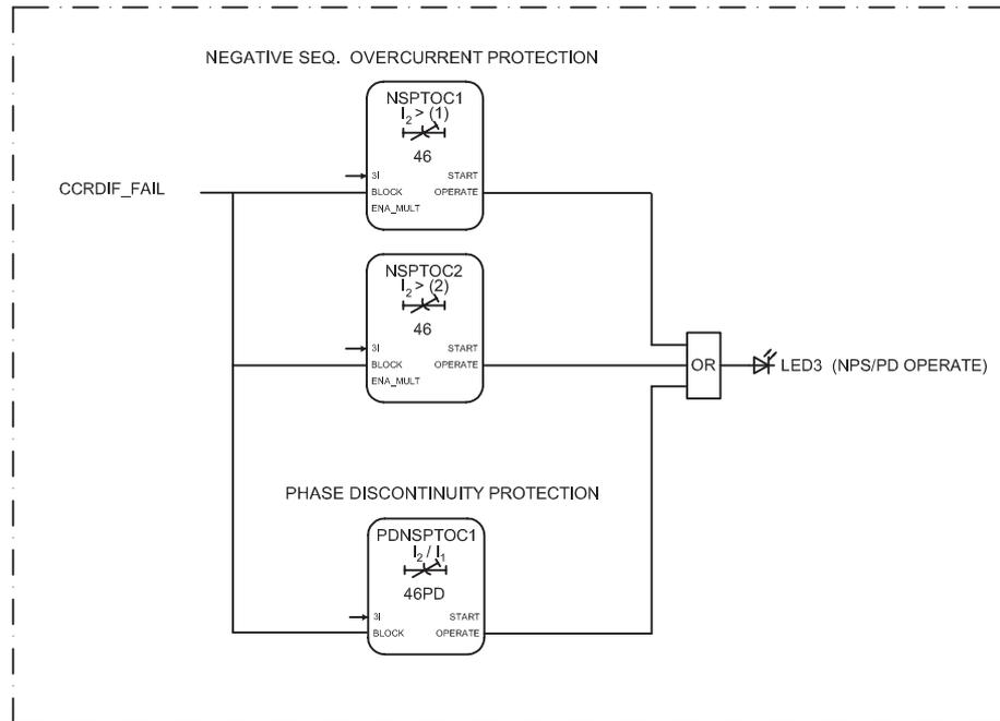
Figure 85: Negative sequence and phase discontinuity protection
