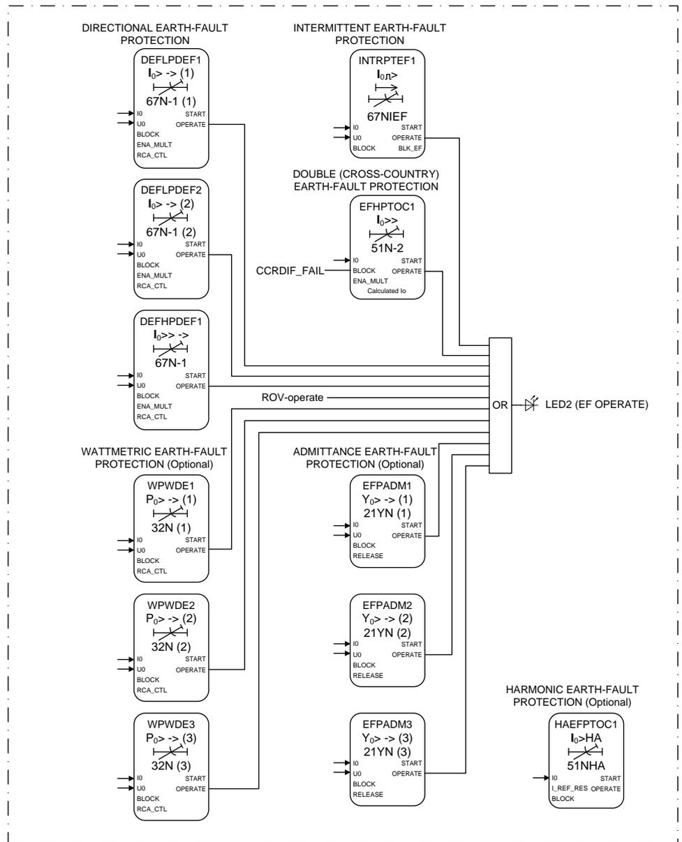
Figure 99: Directional earth-fault protection
