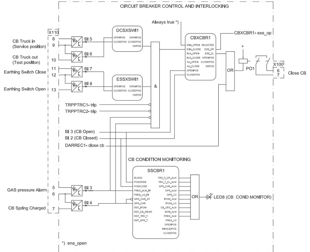
Figure 66: Circuit breaker control
