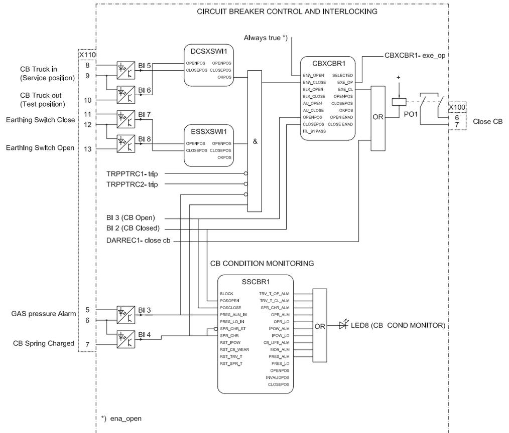
Figure 44: Circuit breaker control
