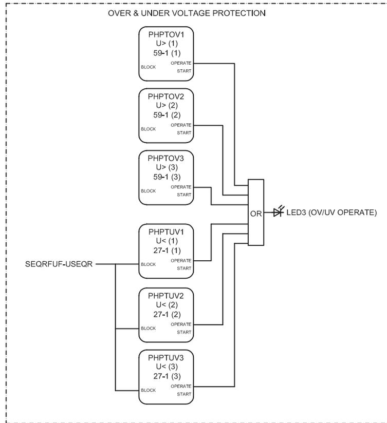
Figure 75: Overvoltage and undervoltage protection
