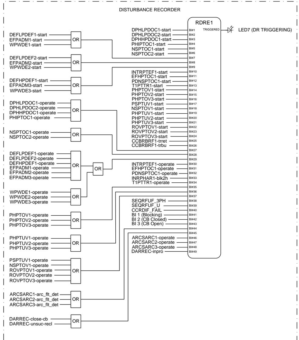
Figure 63: Disturbance recorder
