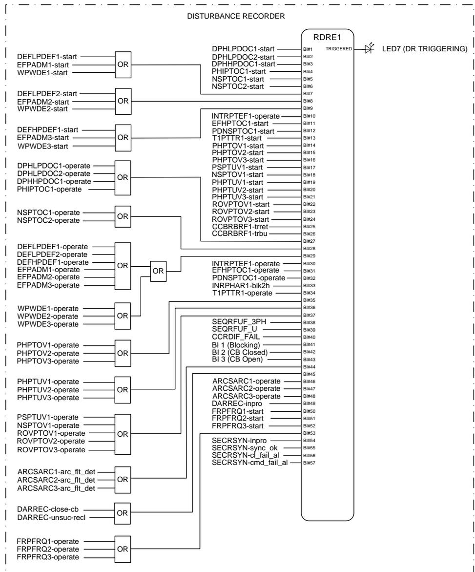
Figure 105: Disturbance recorder
