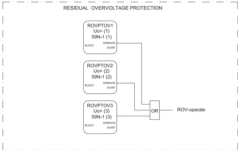
Figure 90: Residual overvoltage protection
