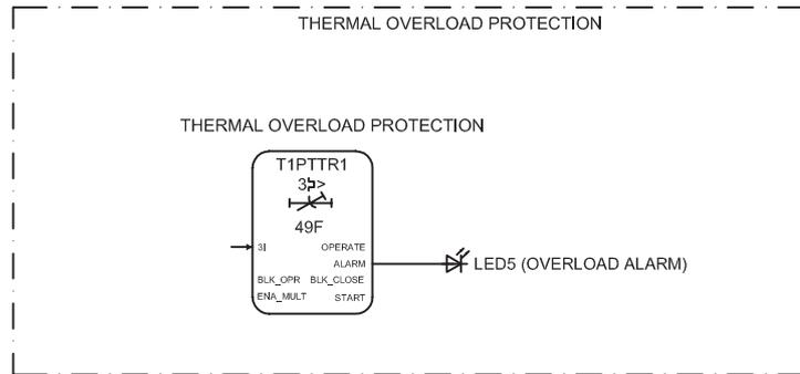
Figure 70: Thermal overload protection
