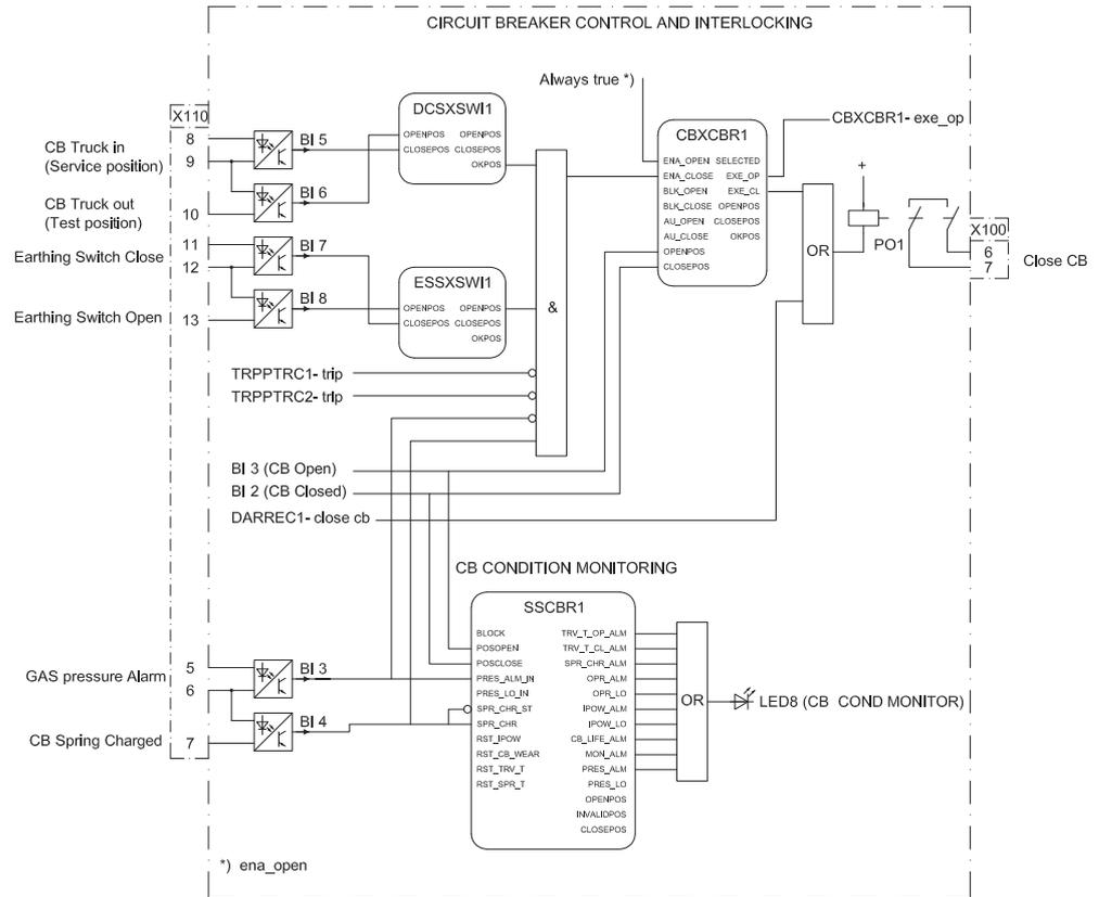
Figure 108: Circuit breaker control
