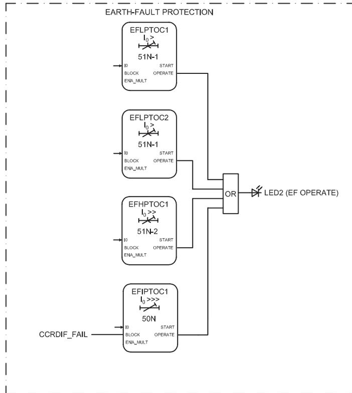
Figure 84: Non-directional earth-fault protection
