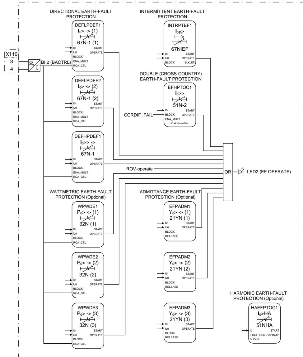
Figure 57: Directional earth-fault protection
