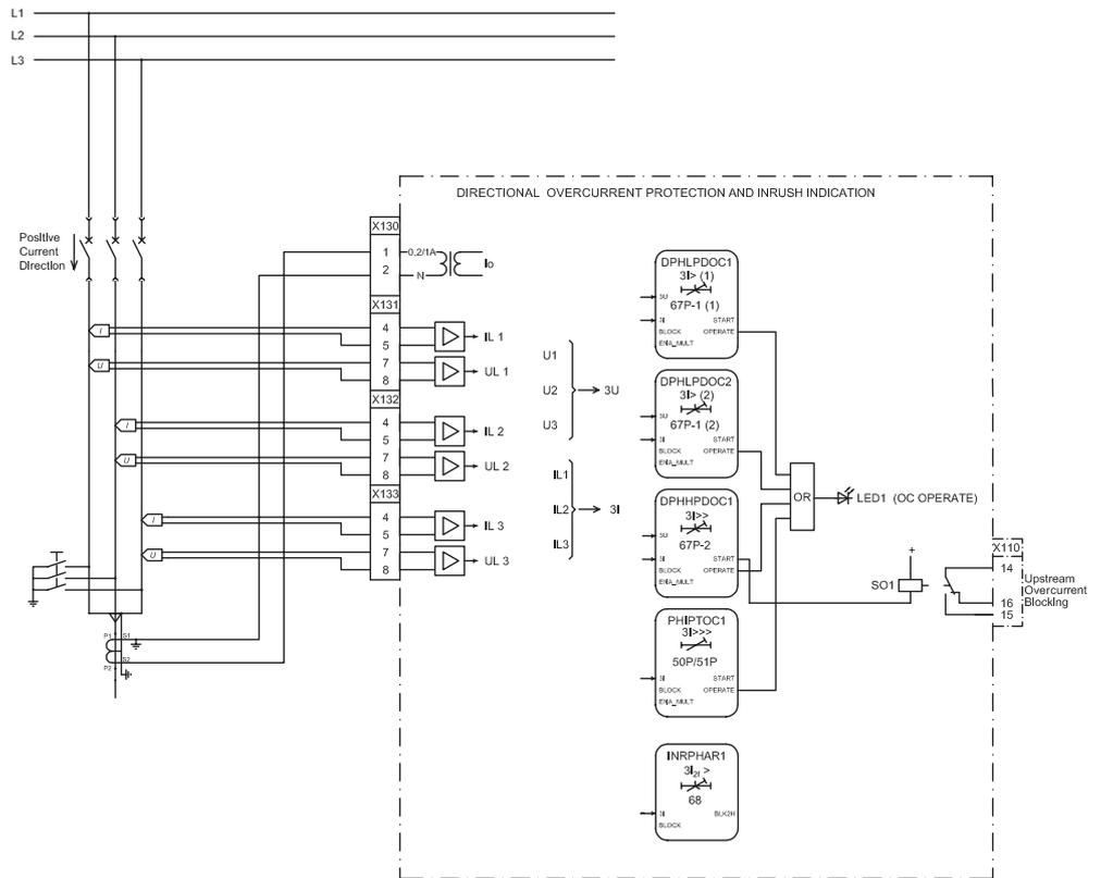
Figure 68: Directional overcurrent protection
