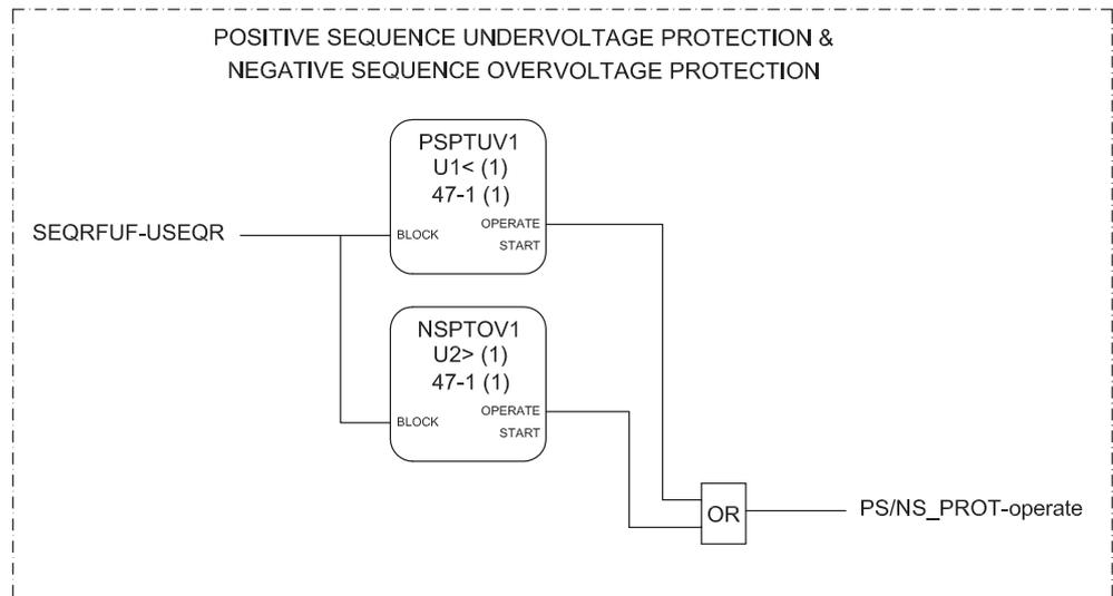
Figure 103: Positive-sequence undervoltage and negative-sequence overvoltage protection
