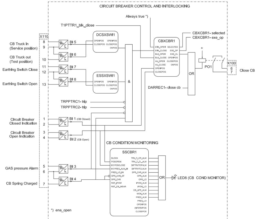
Figure 81: Circuit breaker control
