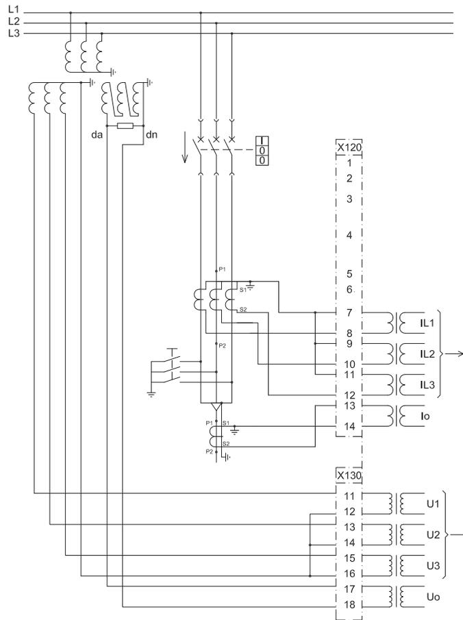
Figure 9: Connection diagram for the E and F configurations
