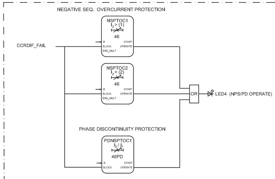
Figure 71: Negative sequence and phase discontinuity protection
