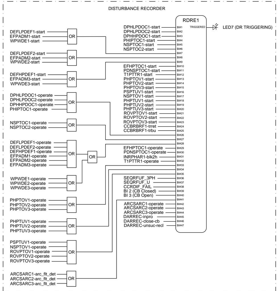
Figure 78: Disturbance recorder
