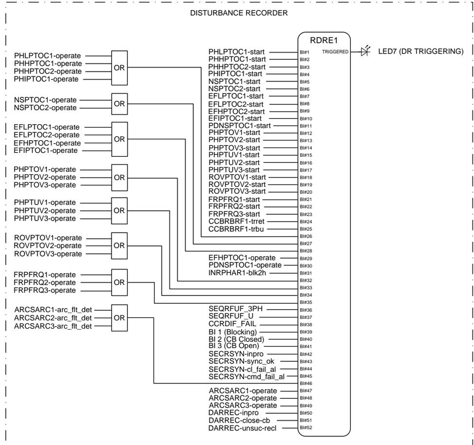
Figure 92: Disturbance recorder
