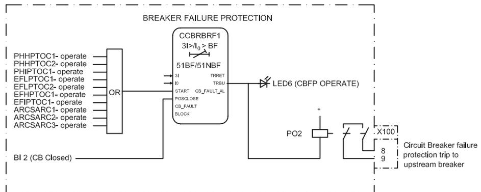
Figure 86: Circuit breaker failure protection
