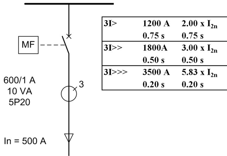
Figure 110: Example of three-stage overcurrent protection
