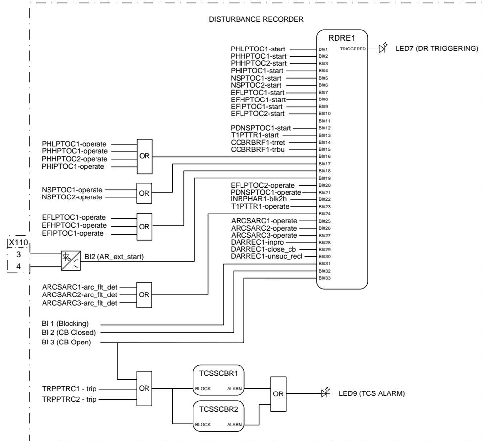
Figure 42: Disturbance recorder
