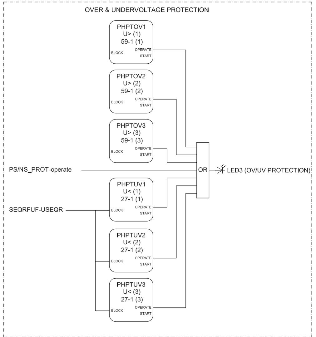
Figure 102: Overvoltage and undervoltage protection
