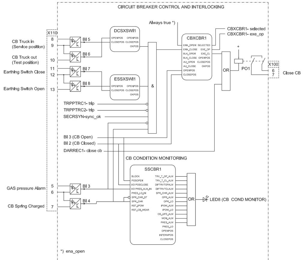
Figure 96: Circuit breaker control
