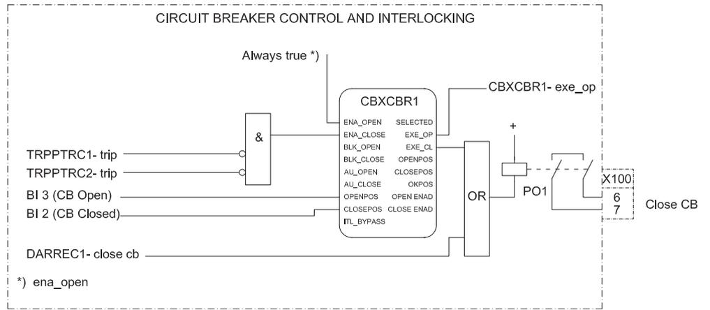
Figure 36: Circuit breaker control
