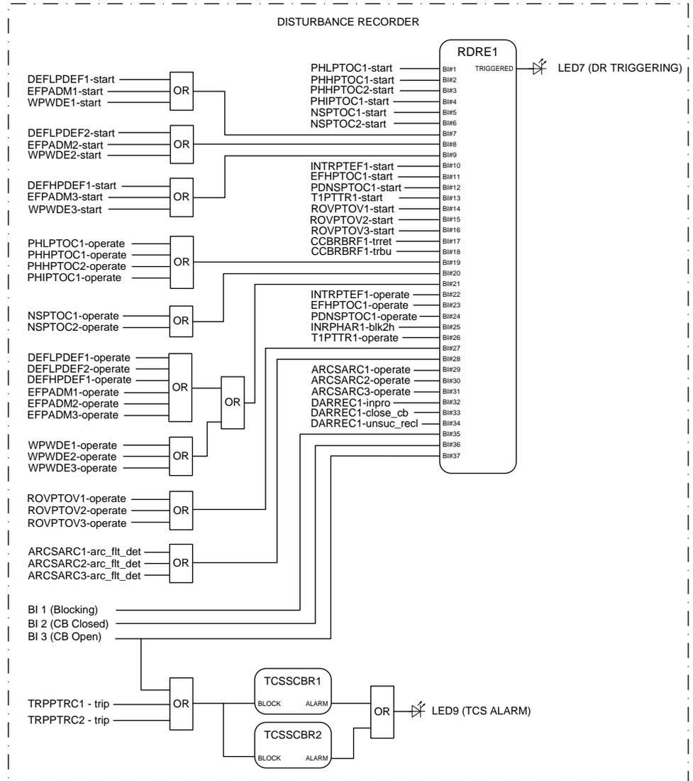
Figure 17: Disturbance recorder
