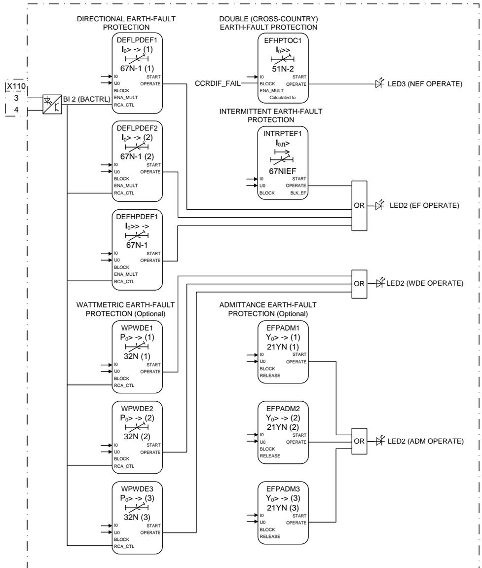
Figure 47: Directional earth-fault protection
