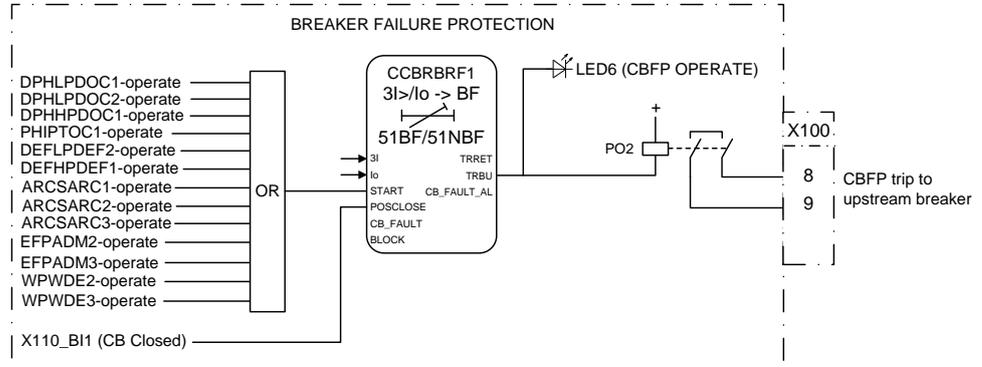
Figure 72: Circuit breaker failure protection
