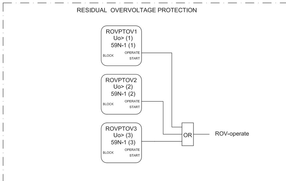
Figure 23: Residual overvoltage protection
