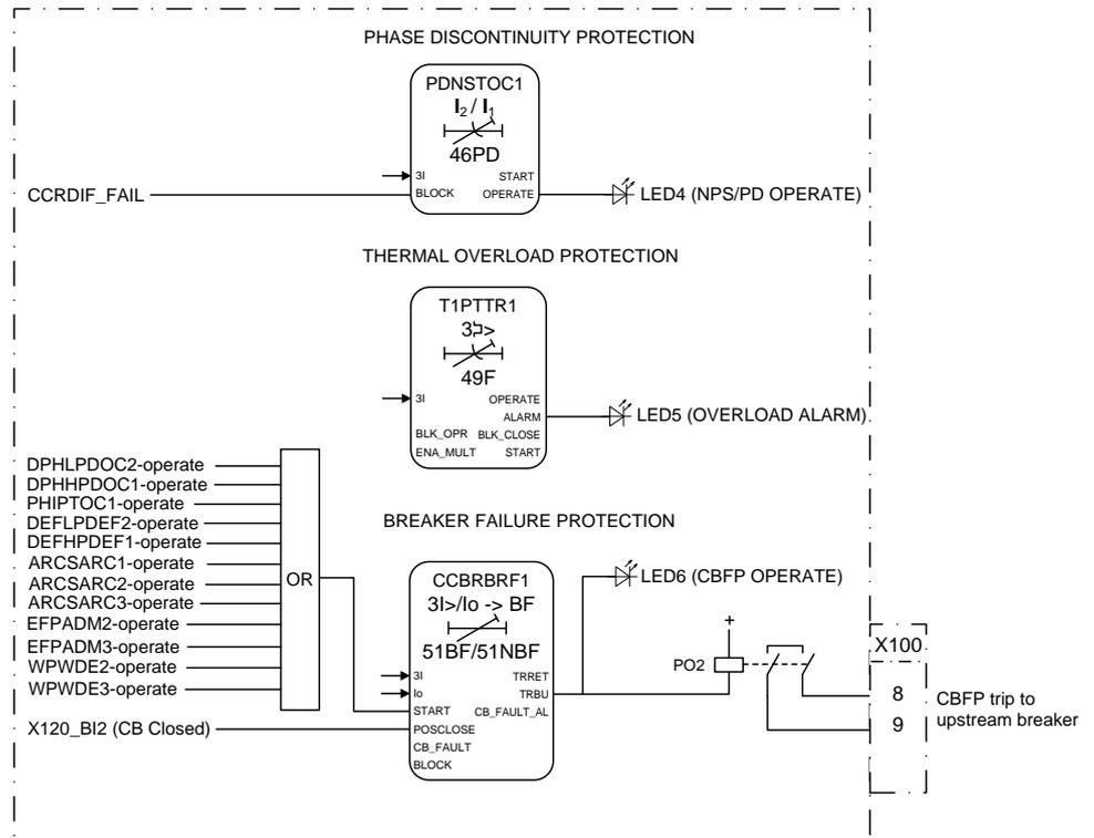
Figure 58: Phase discontinuity, thermal overload and circuit breaker failure protection
