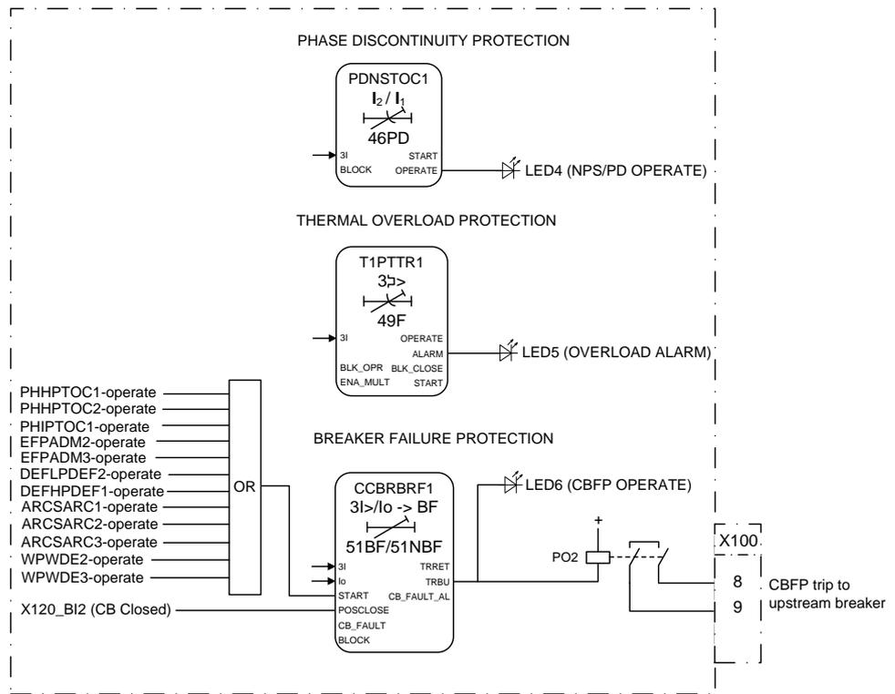
Figure 15: Phase discontinuity, thermal overload and circuit breaker failure protection
