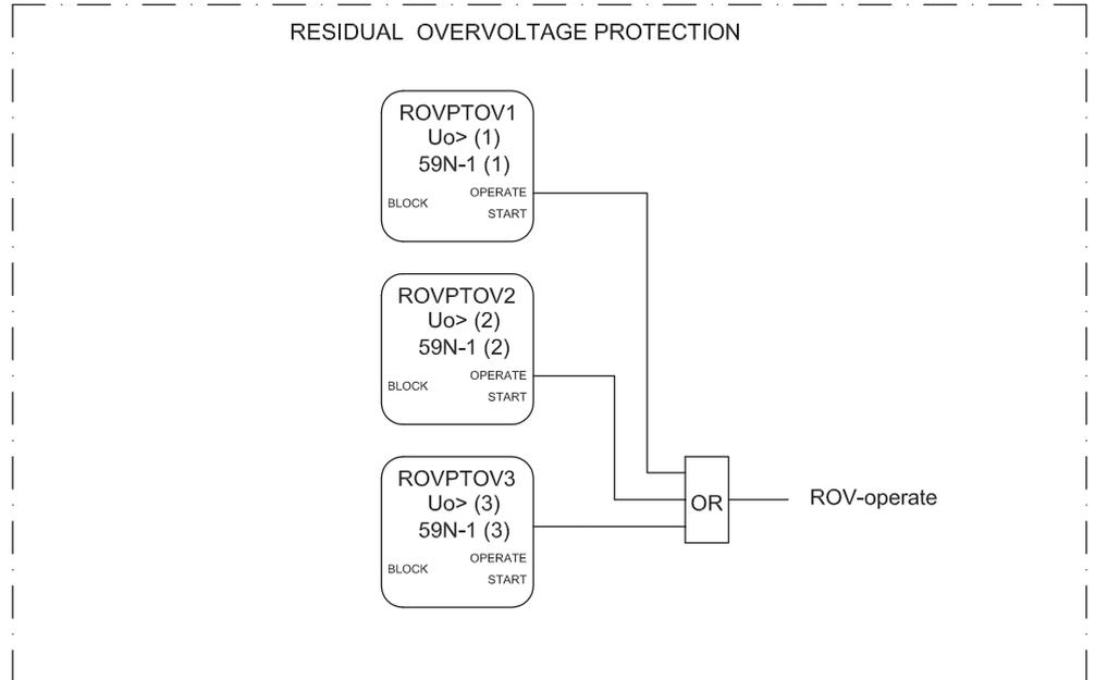
Figure 14: Residual overvoltage protection
