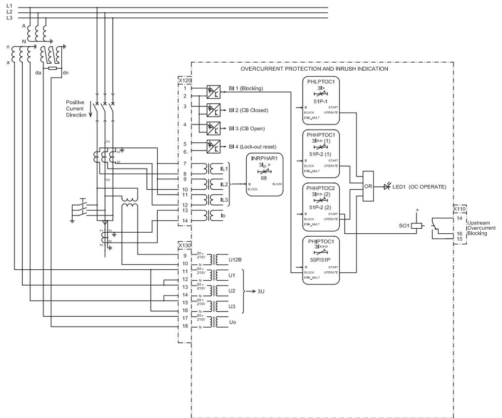
Figure 83: Non-directional overcurrent protection
