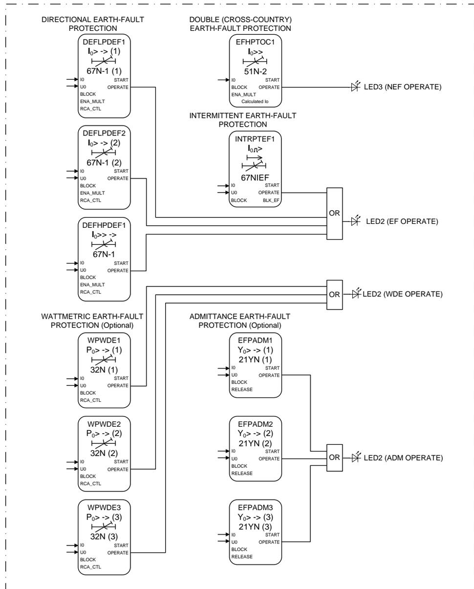
Figure 13: Directional earth-fault protection
