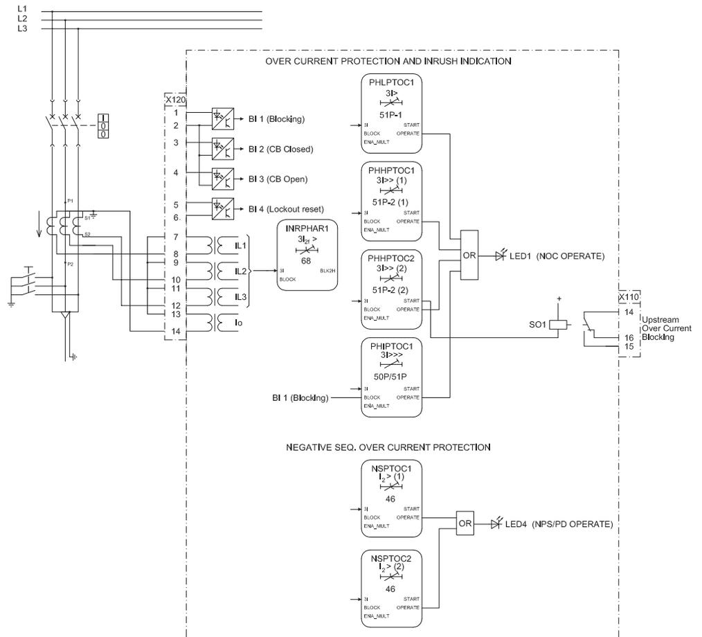
Figure 38: Overcurrent protection
