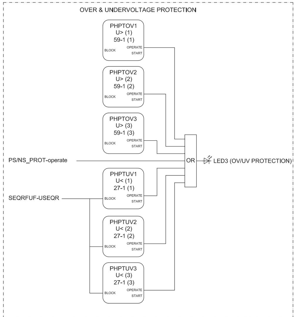
Figure 60: Overvoltage and undervoltage protection
