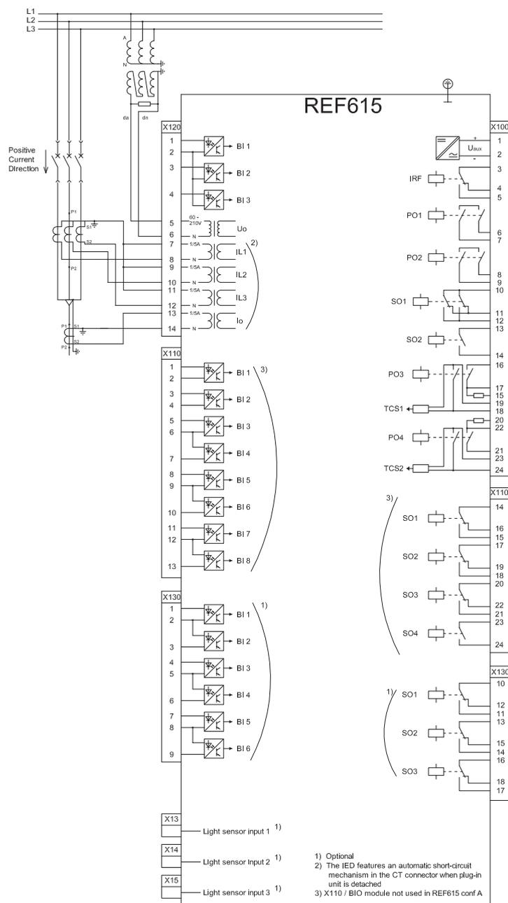
Figure 6: Connection diagram for the A and B configurations<sup>[1]</sup>
