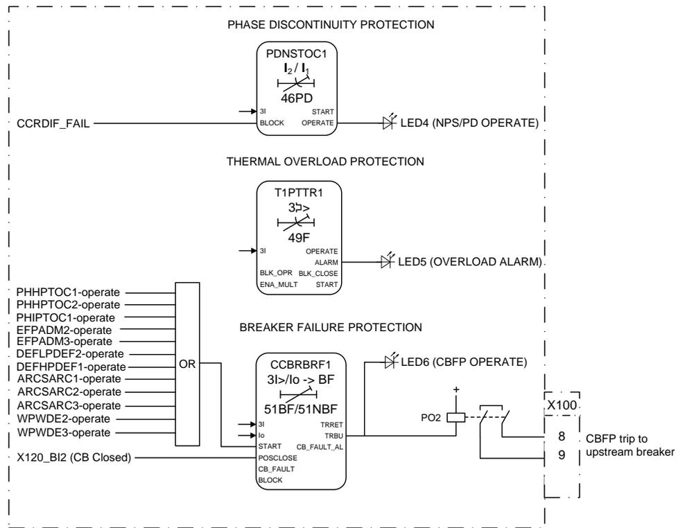
Figure 49: Phase discontinuity, thermal overload and circuit breaker failure protection
