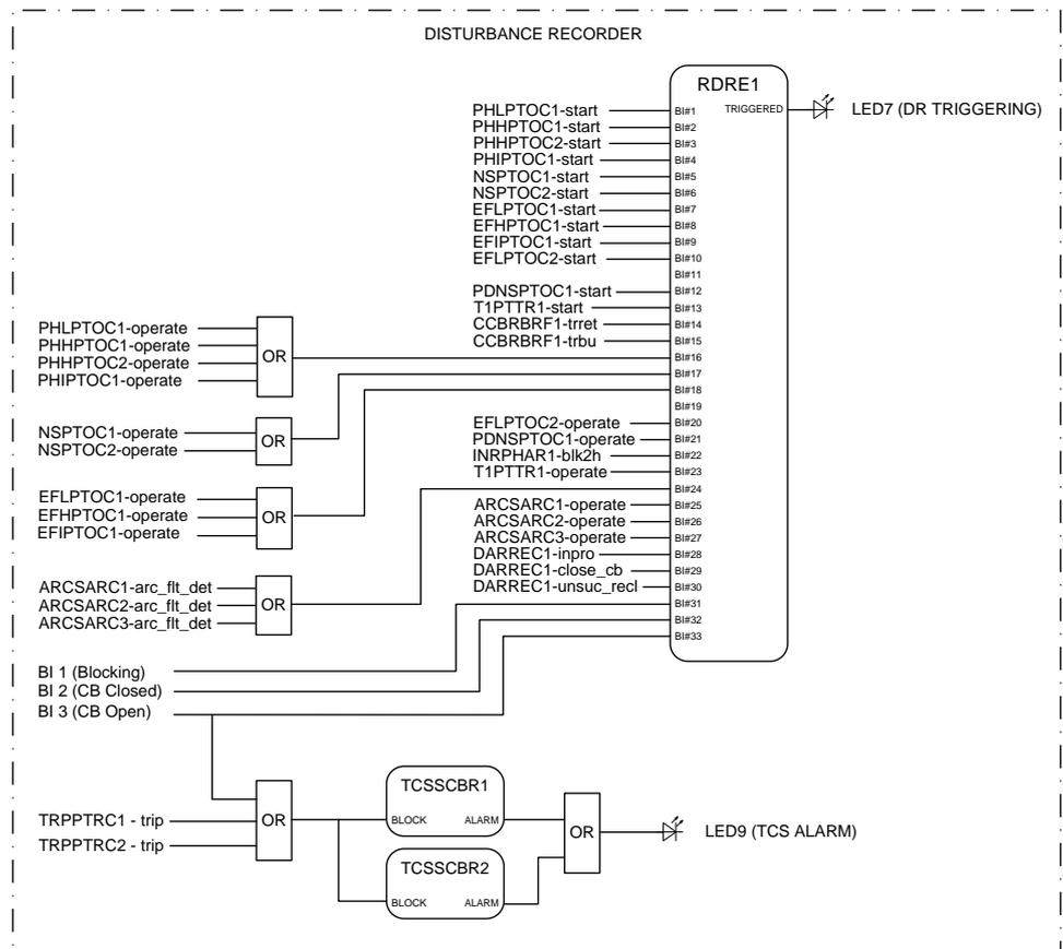
Figure 34: Disturbance recorder
