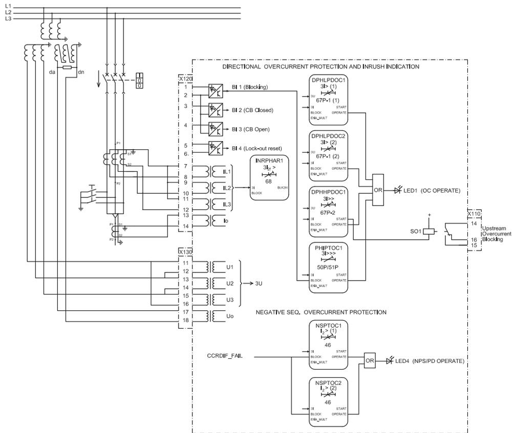
Figure 56: Directional overcurrent protection
