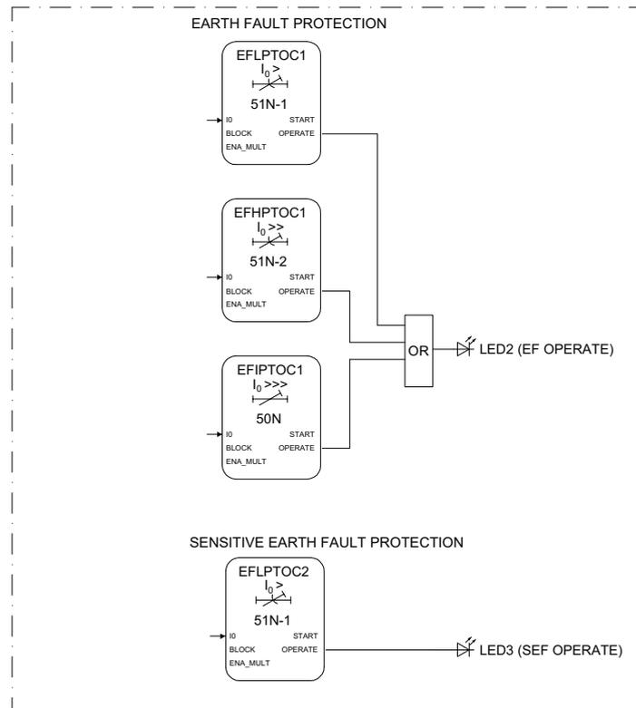
*Figure 31: Non-directional earth-fault protection*
