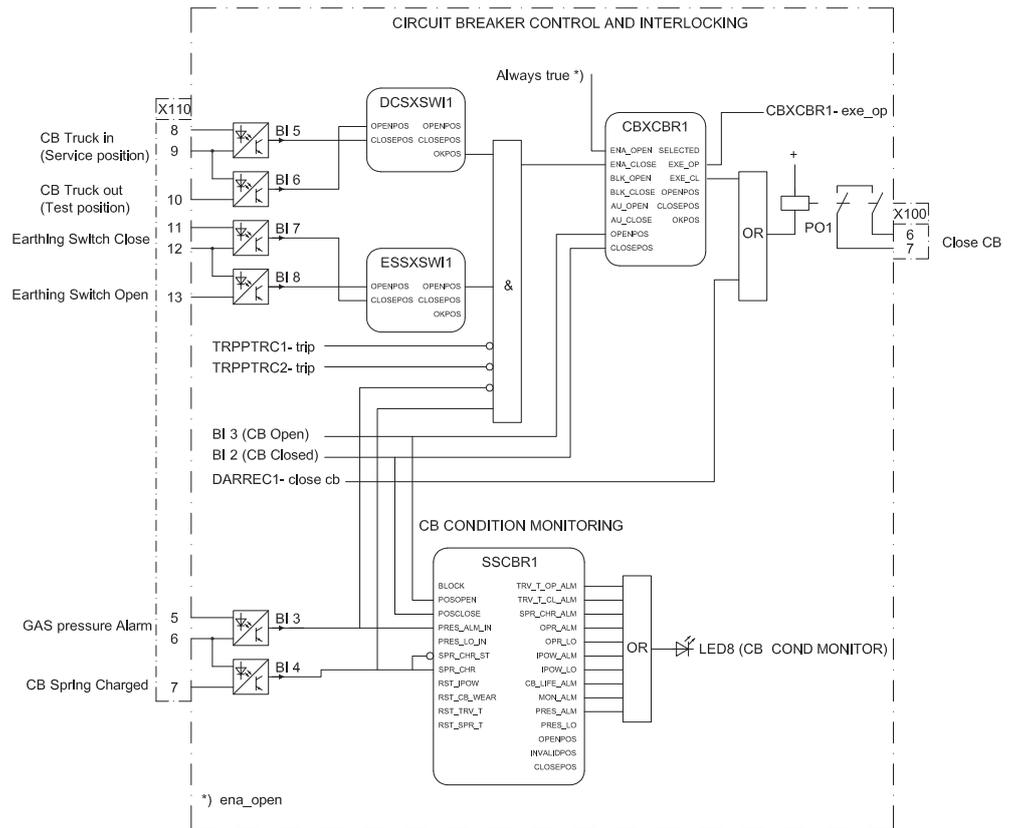
Figure 54: Circuit breaker control
