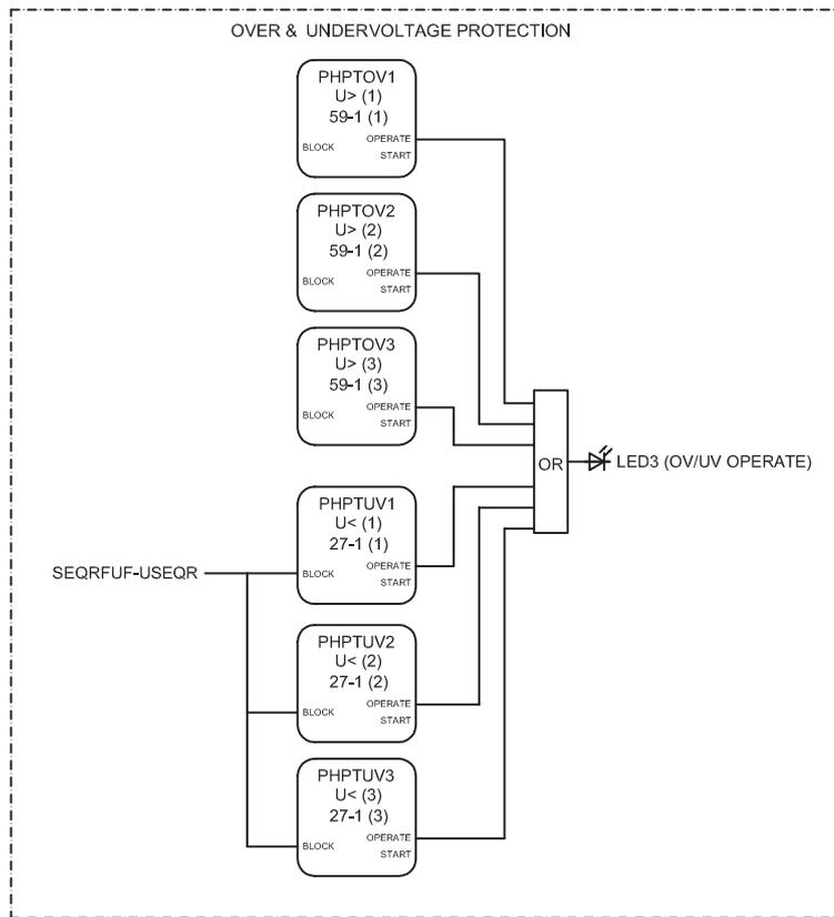
Figure 89: Overvoltage and undervoltage protection
