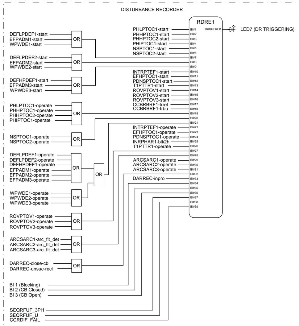
Figure 51: Disturbance recorder
