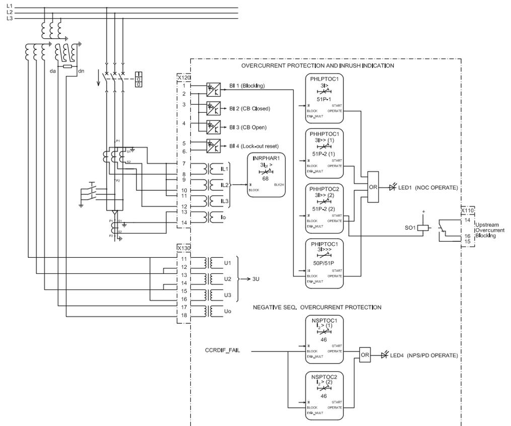
Figure 46: Overcurrent protection
