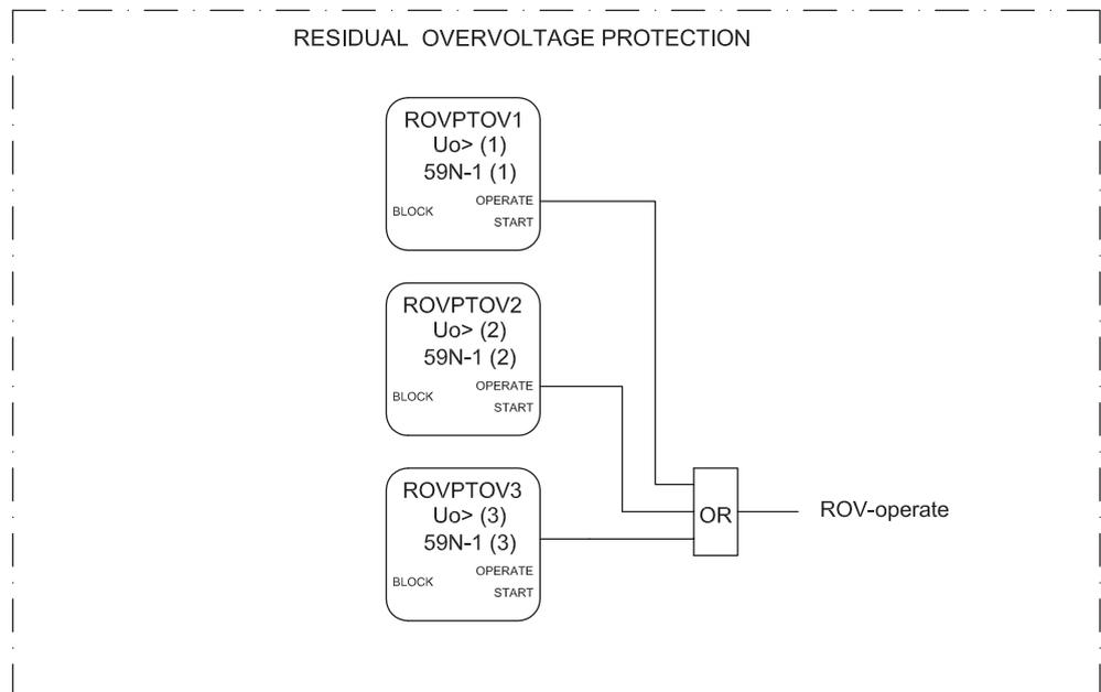
Figure 104: Residual overvoltage protection
