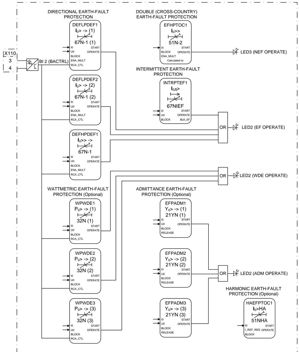
Figure 22: Directional earth-fault protection
