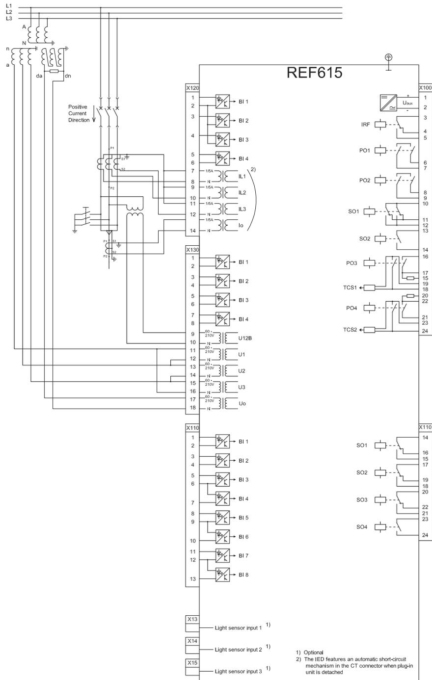
Figure 11: Connection diagram for the H and J configuration
