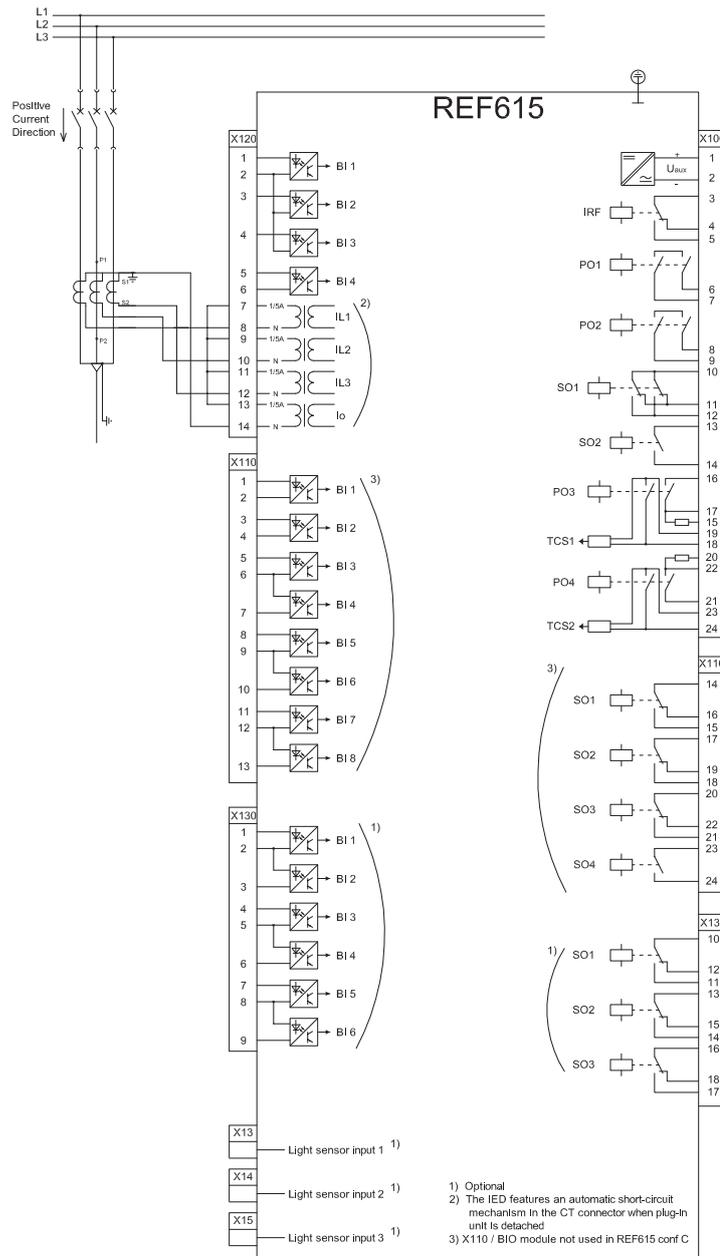
Figure 7: Connection diagram for the C and D configurations [2]
