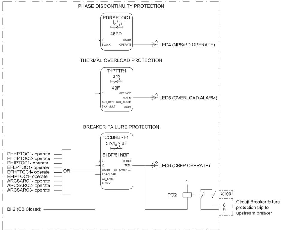
Figure 32: Phase discontinuity, thermal overload and circuit breaker failure protection
