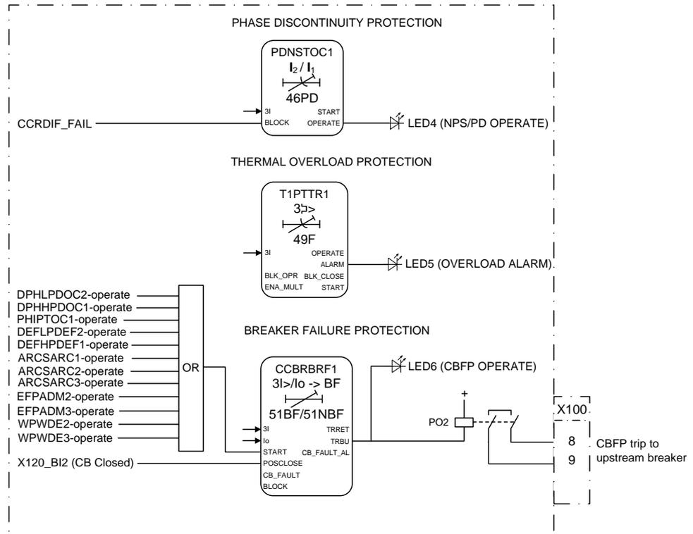
Figure 100: Phase discontinuity, thermal overload and circuit breaker failure protection
