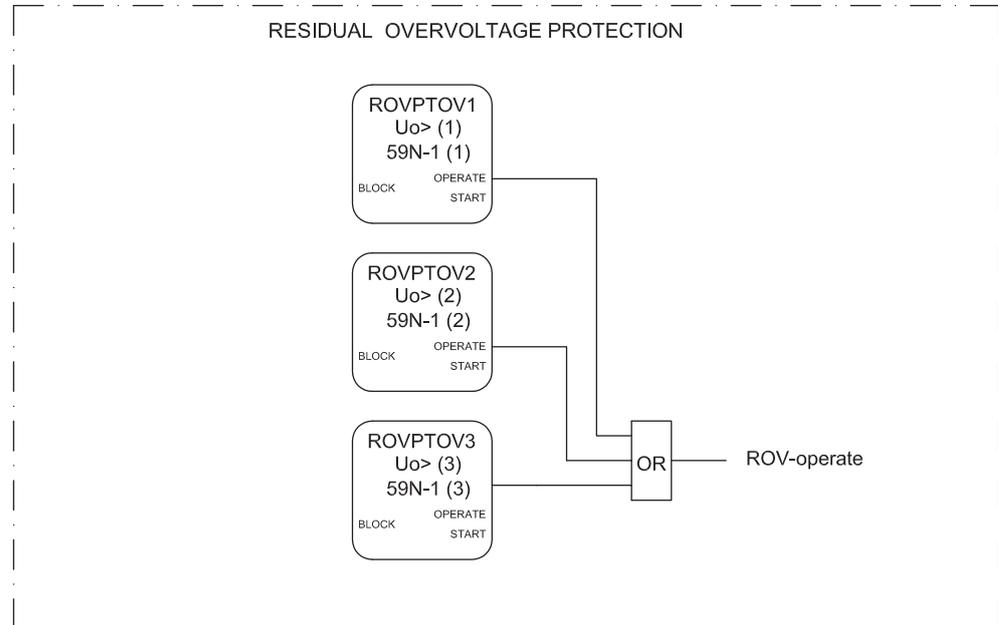
Figure 77: Residual overvoltage protection
