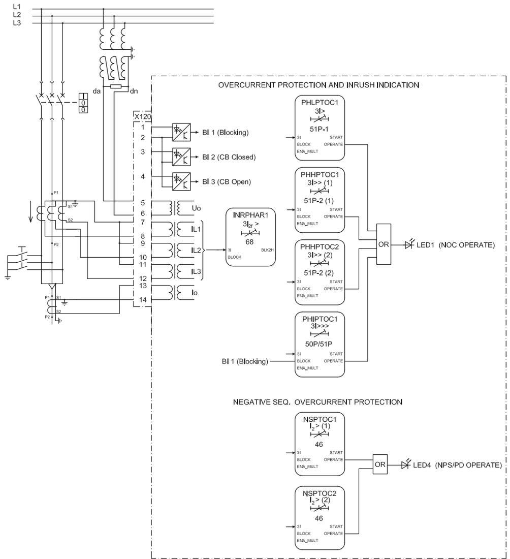
Figure 12: Overcurrent protection
