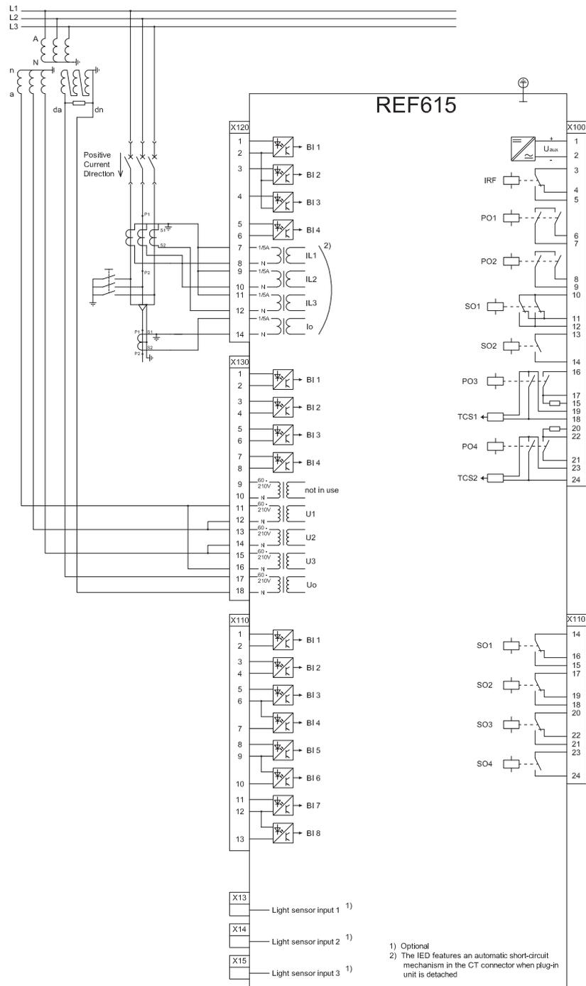
Figure 8: Connection diagram for the E and F configurations
