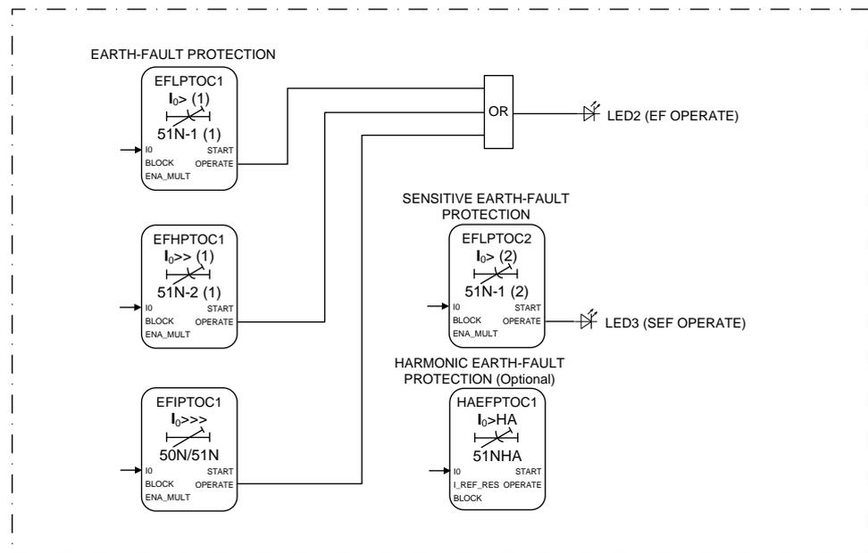
Figure 39: Non-directional earth-fault protection
