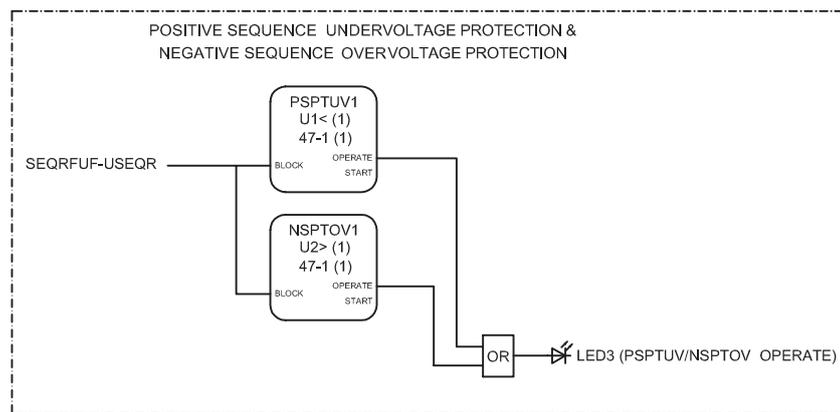
Figure 76: Positive-sequence undervoltage and negative-sequence overvoltage protection
