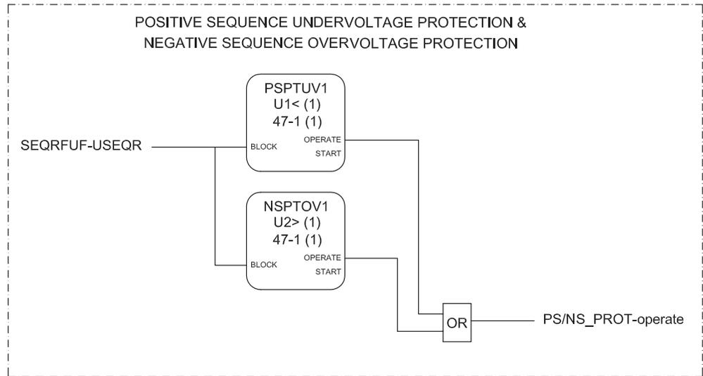
Figure 61: Positive-sequence undervoltage and negative-sequence overvoltage protection
