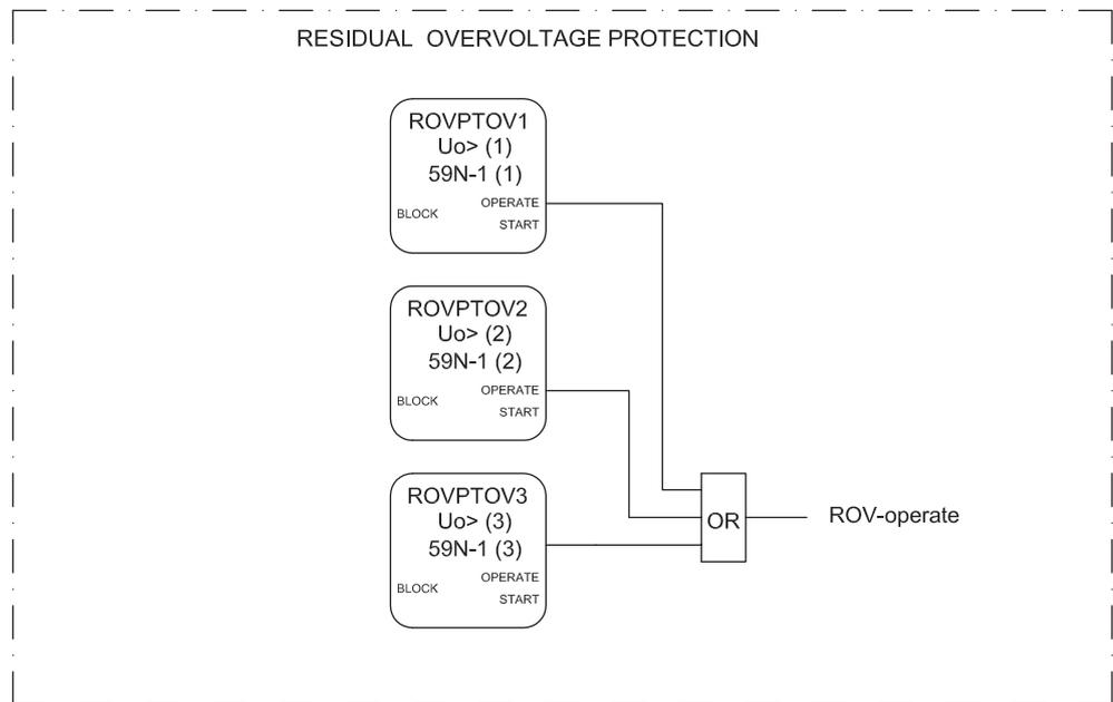
Figure 62: Residual overvoltage protection
