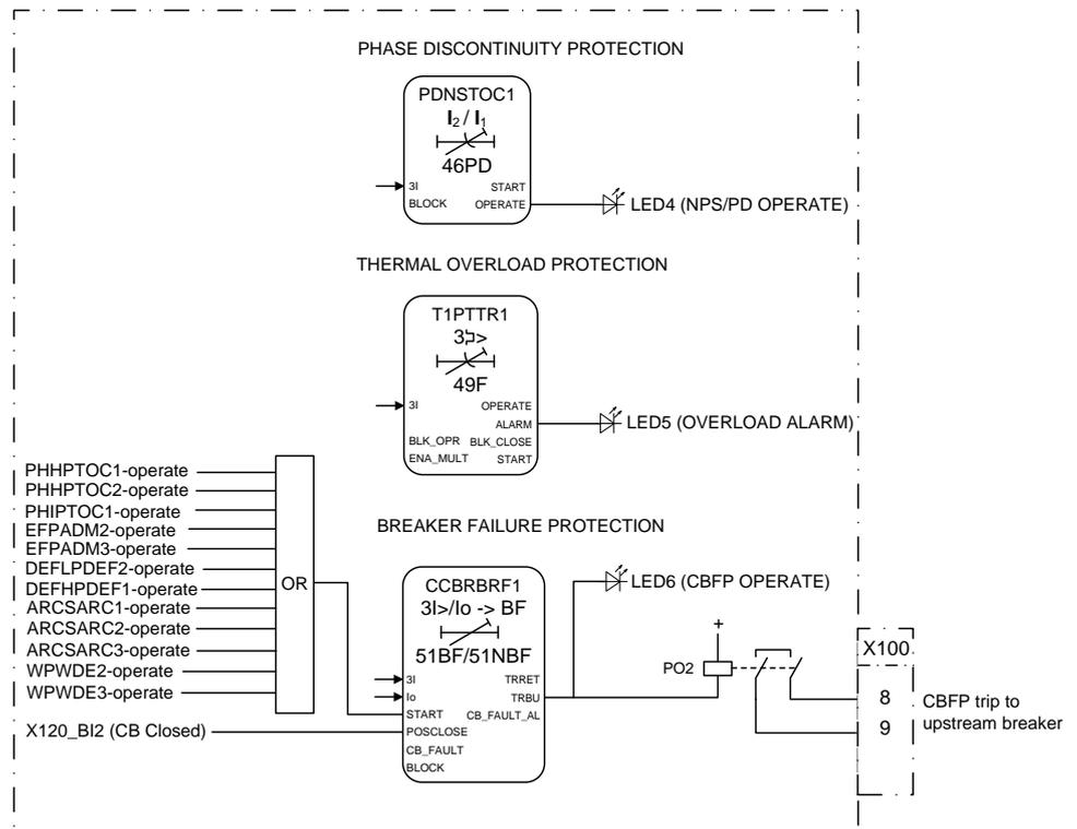
Figure 24: Phase discontinuity, thermal overload and circuit breaker failure protection
