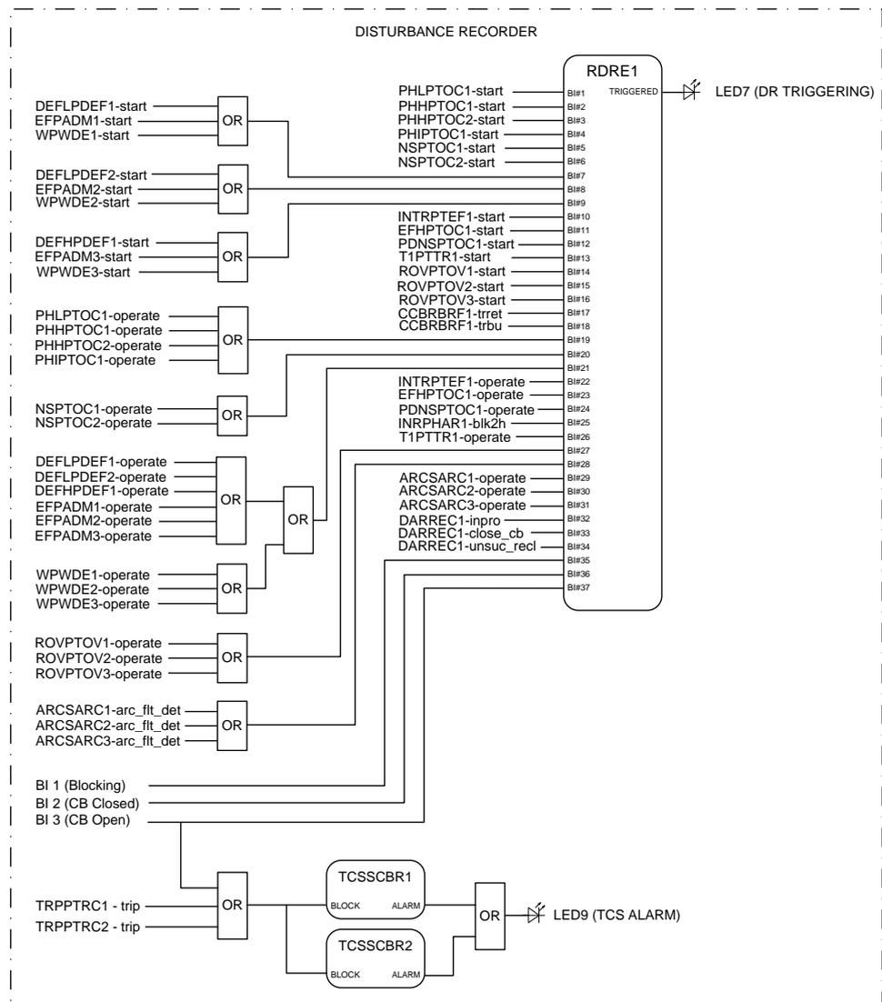
Figure 26: Disturbance recorder
